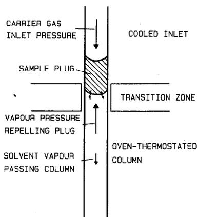
Fig. 2. Solvent evaporation from a stationary sample plug, positioned such that the front of the plug is located at a point where the temperature corresponds to the boiling point of the solvent at the inlet pressure. The plug is kept stationary as the solvent vapour pressure equals the carrier gas inlet pressure.
